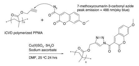
Scheme 1. Click reaction between iCVD pPA and azido functionalized fluorescent dye, N<sub>3</sub>-coumarin.
