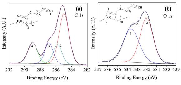
Fig. 2. XPS high resolution scan data of pPA; (a) C 1s and (b) O 1s, respectively.
