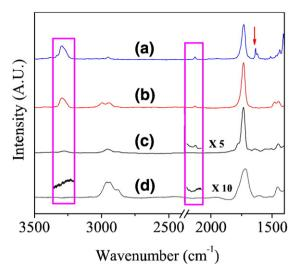
**Fig. 1.** FTIR spectra of (a) PA monomer, (b) iCVD pPA, (c) iCVD p(PA-co-EGDA), and (d) plasma polymerized pPA. Rectangular regions represent C–H stretch in acetylene group (around 3200 cm<sup>-1</sup>) and C=C stretch in acetylene group (around 2100 cm<sup>-1</sup>) and arrow represents C=C stretch in acrylate (around 1600 cm<sup>-1</sup>).
